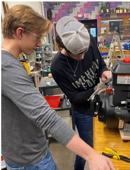
Eli and Nathaniel working to remove the carburetor from this snowmobile engine as a part of the small engines class.
